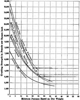
Fig. 13.—Relation between the crushing strength in compression parallel to grain, and the moisture content for several woods.
